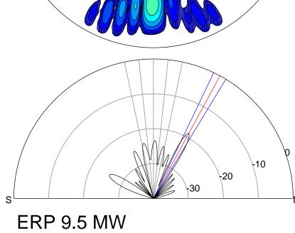
Peak gain 10.1 dBi at Az 359 Zen 28 LHCP gain 20.8 dBi N-S peak 10.1 dBi at Zen 28.4 N-S -3 dB beamwidth 5.6 deg.
