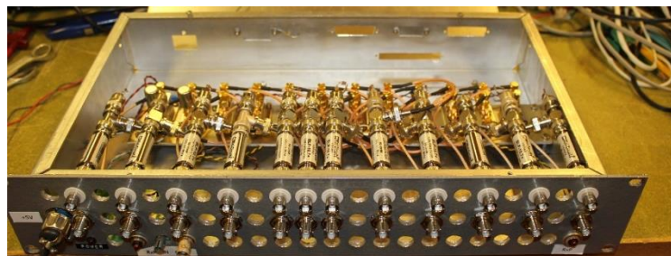
Figure 4. Rack unit containing receiver protectors, low-pass filters and diode clamps.
